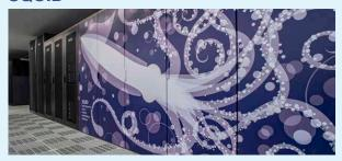
**SQUID** is short for Supercomputer for Quest to Unsolved Interdisciplinary Datascience. SQUID is a new cluster system being operated since May 2021. This system is composed of General purpose CPU nodes, GPU nodes, and Vector nodes, total 1,598 nodes. These nodes and large-scale storage EXAScaler (Lustre 21.2 PB) are interconnected on InfiniBand HDR (200 Gbps) and form a cluster.
