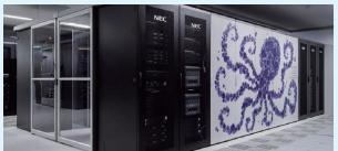
**OCTOPUS** is short for Osaka university Cybermedia cenTer Over-Petascale Universal Supercomputer. OCTOPUS is a cluster system being operated since December 2017. This system is composed of General purpose CPU nodes, GPU nodes, Large-scale shared-memory nodes, and Xeon Phi nodes, total 319 nodes. These nodes and large-scale storage EXAScaler (Lustre 3.1 PB) are interconnected on InfiniBand EDR (100 Gbps) and form a cluster.
