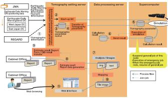
The functionality with which the system stops running jobs, runs this emergency job and then recovers the previous running jobs to the original status heavily depends on NEC NQSII/JM, the proprietary job scheduler proprietary from NEC
