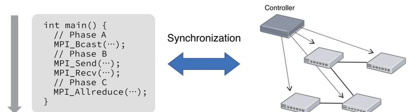
Encode the MPI envelope into a tag and embed into each packet in the kernel
