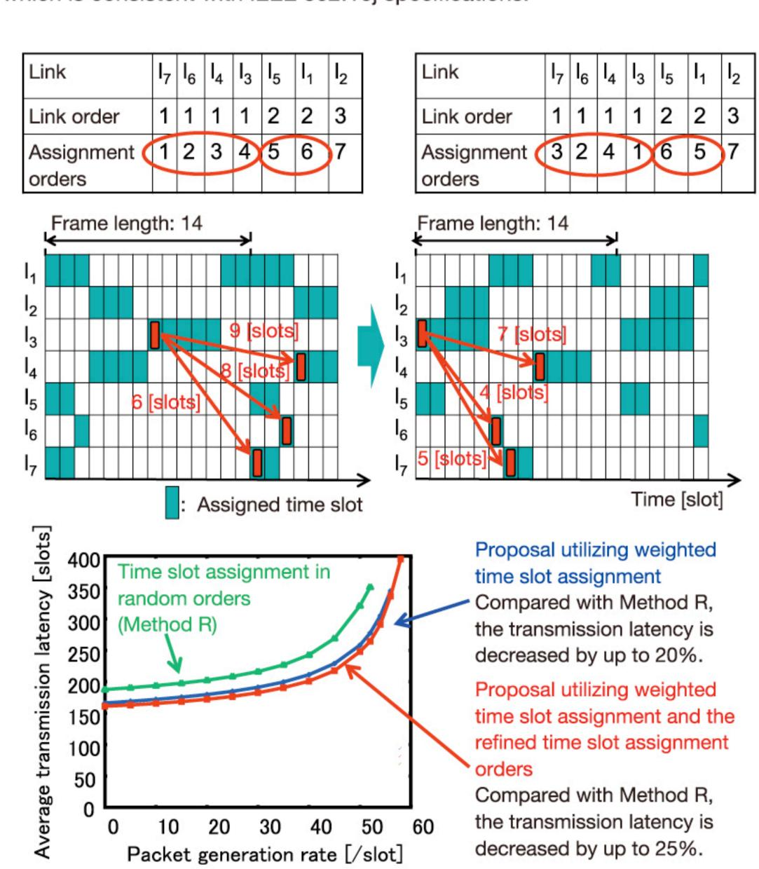
When closely located links in a wireless network are used simultaneously, a receiver node cannot correctly receive radio signals from the corresponding sender node because of radio interference. In time division multiple access (TDMA) protocols, time is divided into frames, each frame consists of time slots of a constant duration, and different time slots are assigned to links that interfere with each other.
