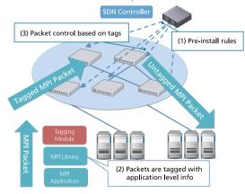
Our implementation embeds a tag into the L2 header. The figure below illustrates the packet tagging mechanism.
