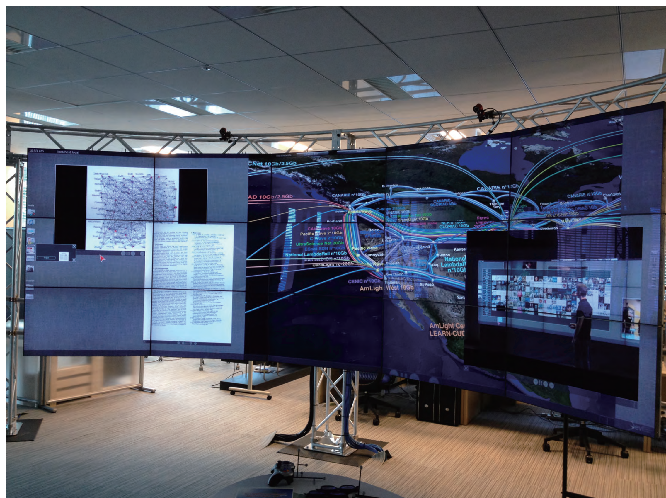
15-screen Cylindrical Stereo Visualization System @ Umekita Office
