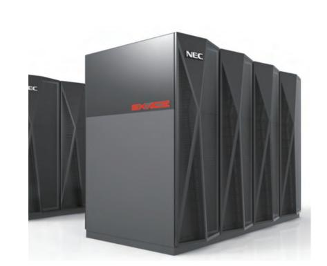
Type: Vector OS: Super-UX # of nodes: 1536 # of cores: 6144 Total memory: 96 TB Peak performance: 423 TFlops
