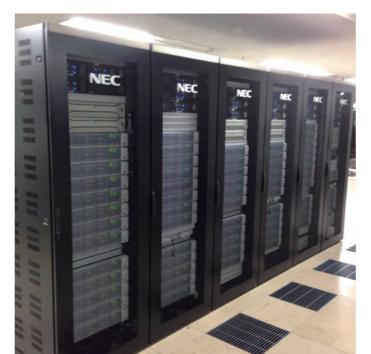
Type: Scalar OS: Linux # of nodes: 56 # of cores: 1120 Total memory: 3.584 TB Peak performance: 22.4 TFlops Accelerator: NVIDIA Tesla K20 × 48
