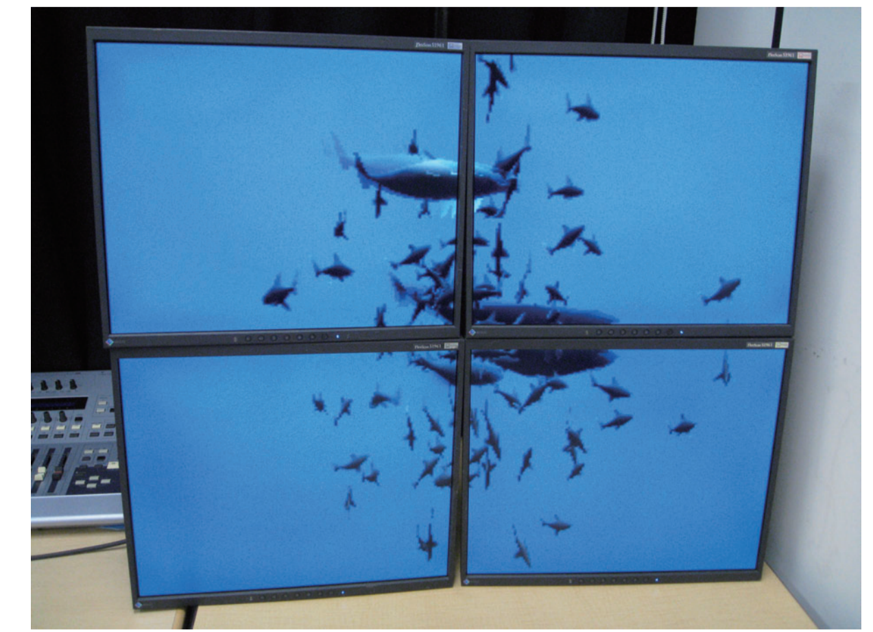
Fig.1 Tiled Display Wall
