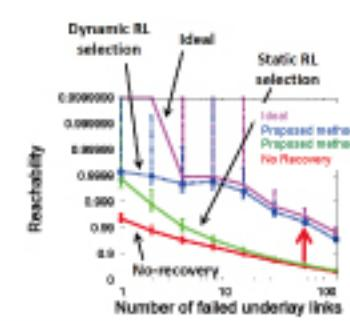
We can improve reachability of the overlay network from 69% to 93%, when 5% links in the underlay network fail simultaneously.
