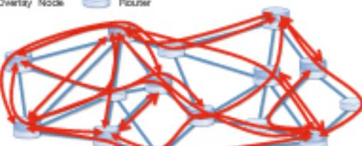
Failure recovery: Since overlay networks share underlay network equipments, a single network failure would bring multiple, simultaneous failures in overlay networks. So, we need failure recovery method from simultaneous failures in overlay networks.
